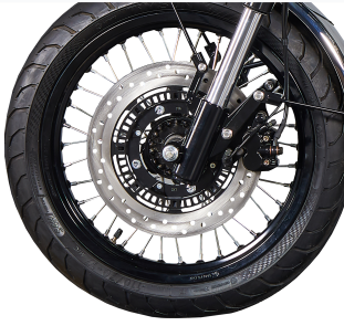
Front assembly featuring spoked wheels, disc brakes, and high-performance tires.
