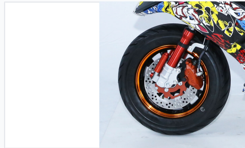
Front wheel assembly featuring a hydraulic disc brake and orange rim.
