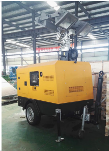
Mobile generator unit mounted on a trailer, featuring integrated floodlights for outdoor and emergency deployment.
