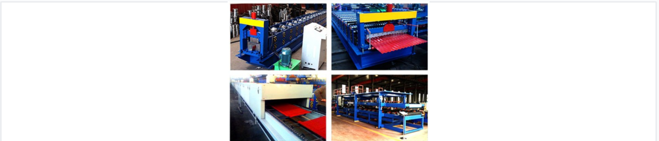
Complete workflow from decoiler to roll forming and outfeed conveyor.
