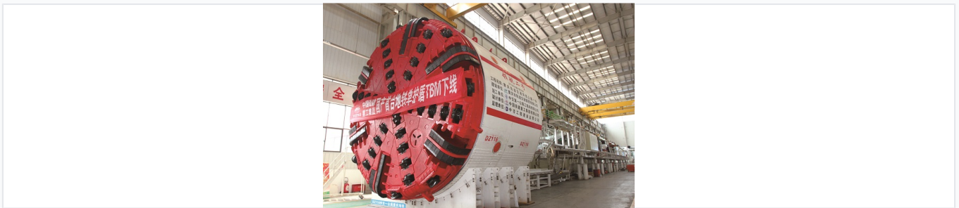
A single shield TBM designed for efficient excavation and segment lining in complex geological conditions.
