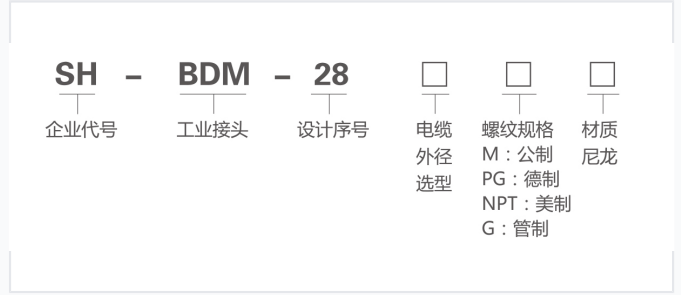
Reference chart for identifying thread standards and model sizing.
