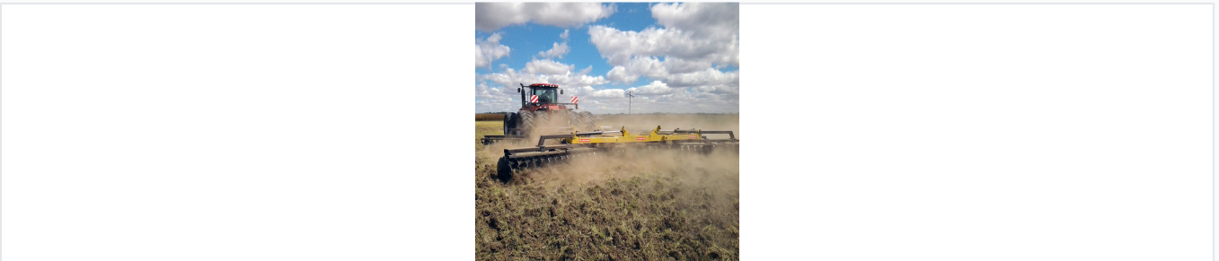
The heavy duty disc harrow deployed for primary tillage and seedbed preparation.
