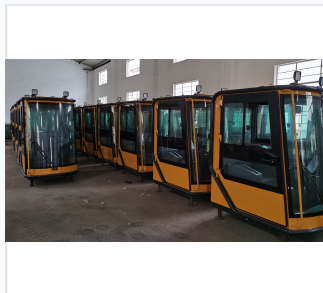
Fully enclosed cabin design featuring integrated safety glass and pre-wired electrical provisions.
