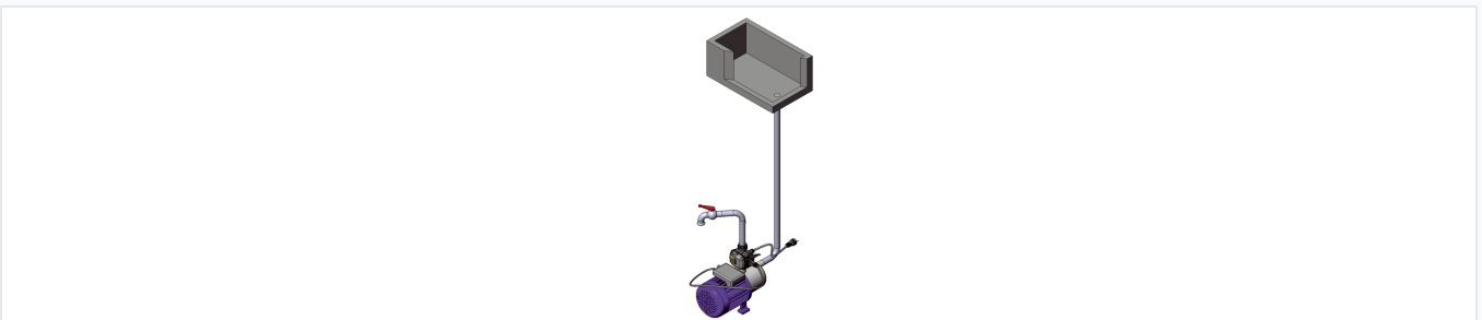
Typical installation of the flow switch within a booster pump system.
