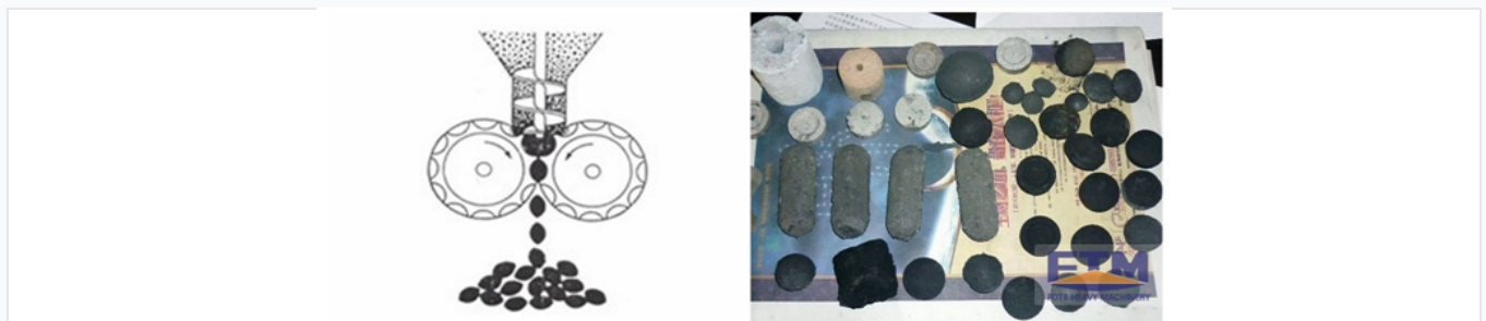
The machine features a robust feeding mechanism and counter-rotating rollers to ensure consistent briquette density.
