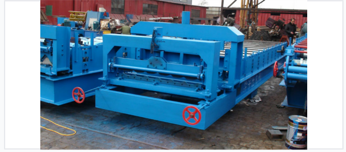
Manual adjustment mechanisms allow for precise coil positioning and tension control.
