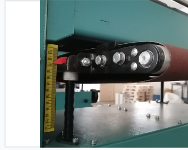
Precision height adjustment system with a visual linear scale for repeatable thickness settings.
