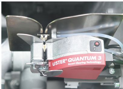
Advanced sensor head for detecting and removing yarn defects during the winding process.
