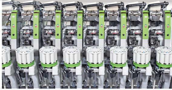
Close-up of the winding heads equipped with precision tension control and anti-patterning mechanisms.
