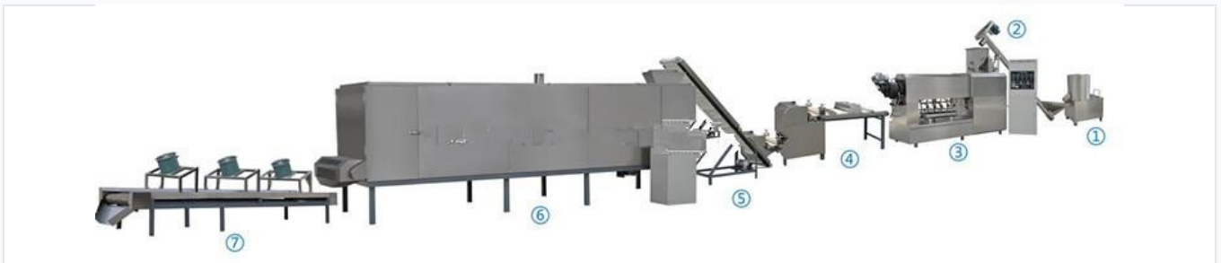
A complete view of the integrated macaroni production line from mixing to drying.
