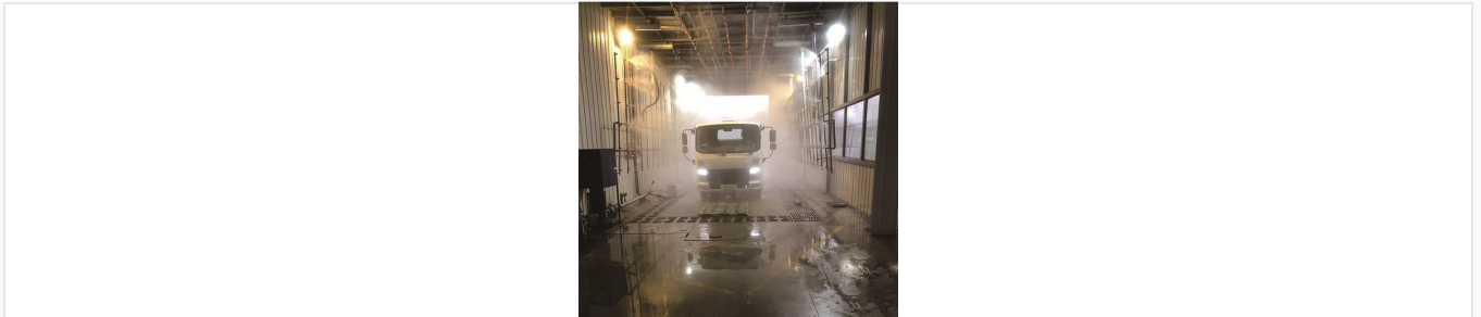
Pre-delivery rain and wash testing to verify cabin sealing and electrical protection.
