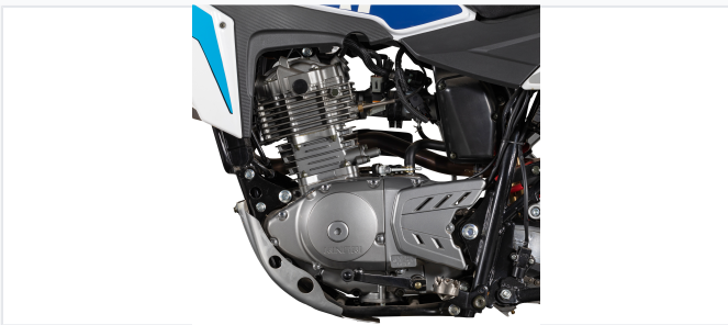
High performance 200cc oil-cooled engine configuration.
