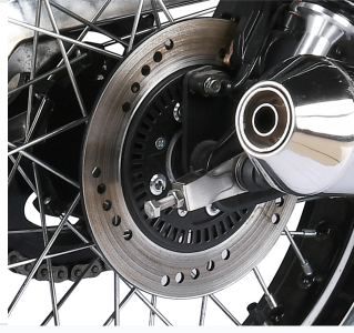
Detailed view of the drilled brake disc, stainless steel muffler, and adjustable suspension.
