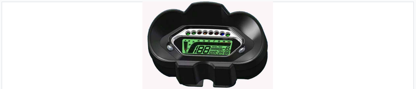
Modern digital instrument cluster displaying speed, RPM, and fuel levels with green backlighting.
